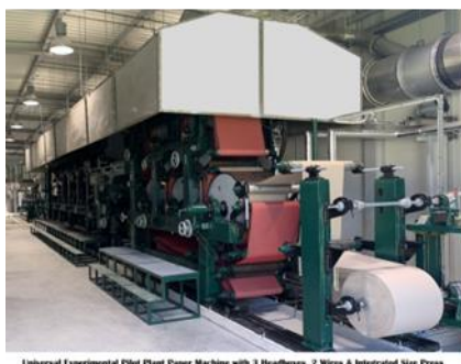
Universal Experimental Pilot Plant Paper Machine with 3 Headboxes, 2 Wires & Integrated Size Press
